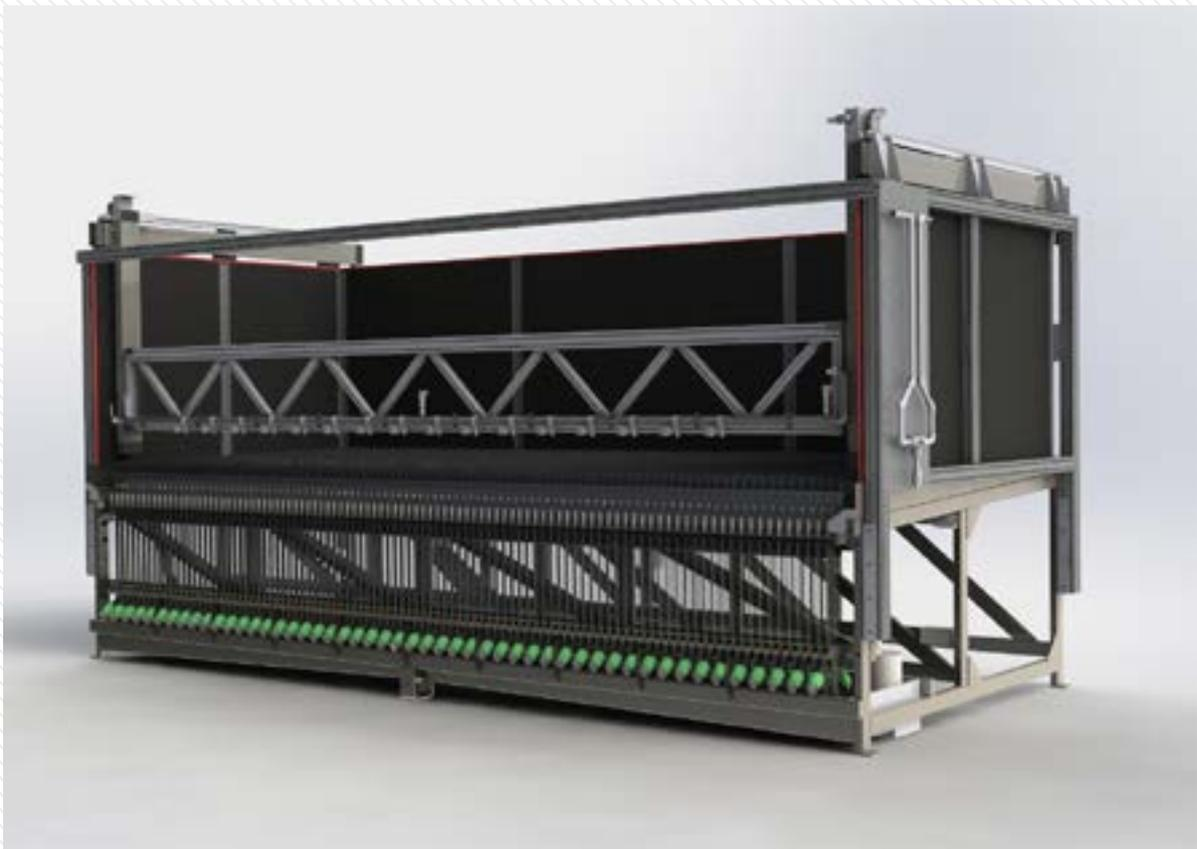
*3d model of a horizontal patternator*
